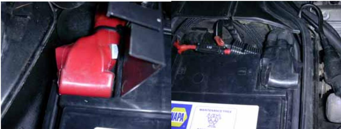
**Image 25 - Red and black rubber boots for the battery clamps**
