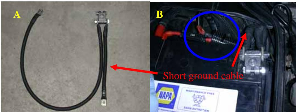
**Image 12 - Battery negative cable and clamp orientation. In B the blue circle highlights the plastic loom covering the accessory positives connecting to the supplemental positive passed the 150 amp fuse.**
