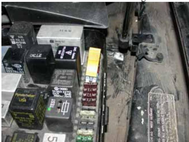
**Image 1 - Removing the fuel pump fuse at #34**
