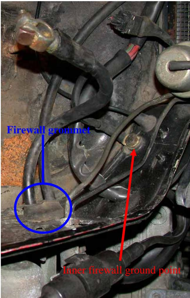
**Image 11 - Inner firewall ground point and grommet**
