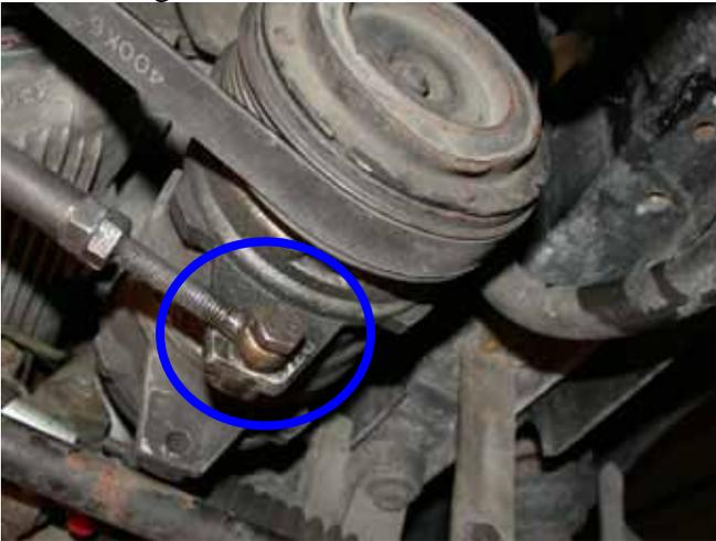
**Image 13 - A/C compressor turnbuckle bolt**
