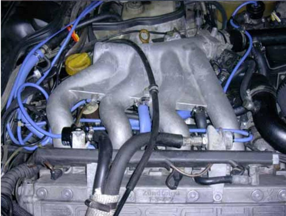
**Image 6 - Intake manifold mounting bolts and vacuum hoses**
